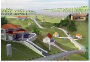
Connecting one or more pump stations to the municipal sewage network can pose distinct challenges depending on the lay of the land. Large pipes of conventional gravity systems need to be laid on a grade. Smaller pipes used for pressure sewage systems don't. This drastically cuts costs associated with excavation and construction of gravity-flow pipelines compared to gravity flow pipe lines.
