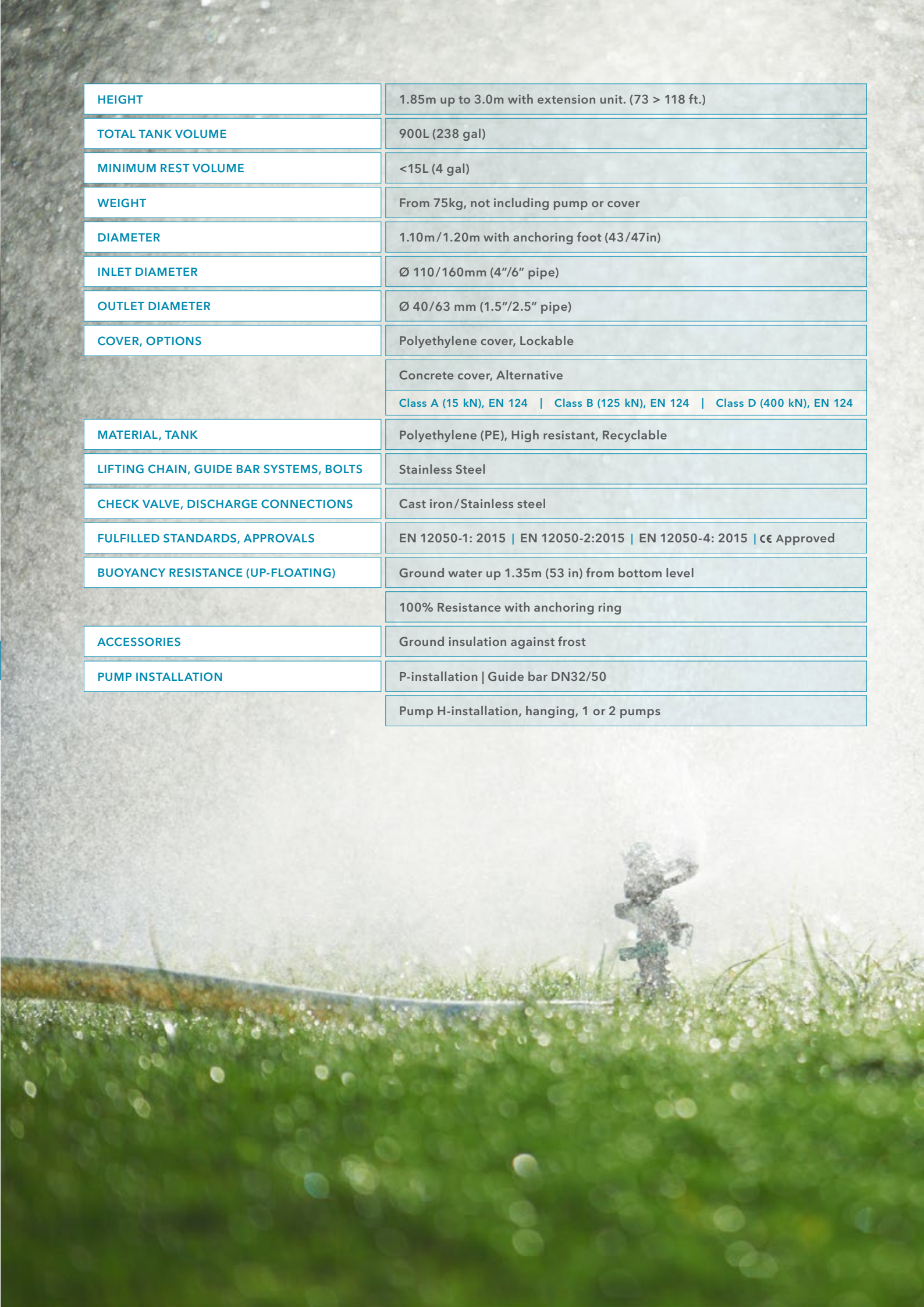
Compit 901 offers hanging installation, H, or guide bar-supported P installation
